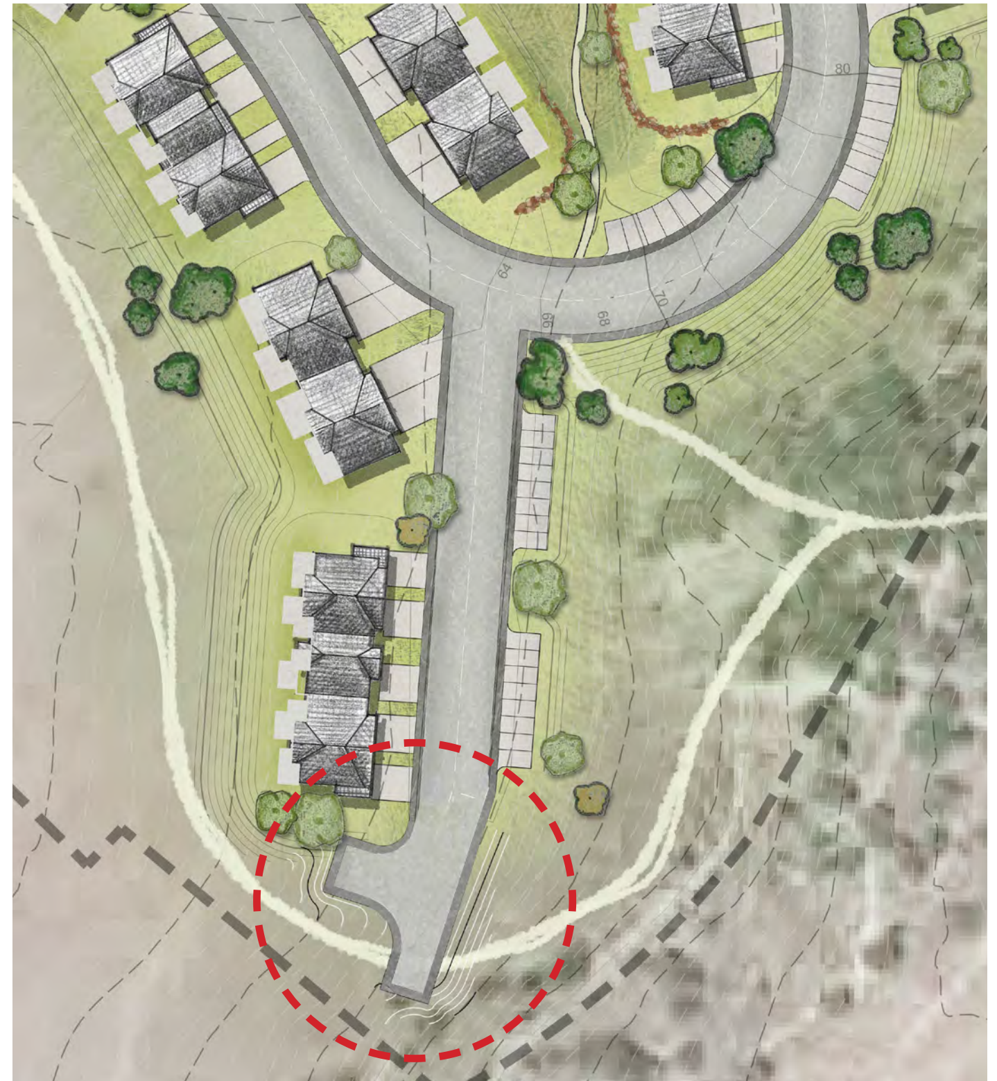
south area alternate emergency 't' turn
